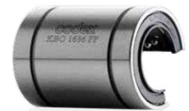
C) OPEN TYPE KBO these units have an opening that corresponds to a single recirculating channel (50 to 100 deg.) Units are used in conjunction with long shafts that are typically supported along the entire length to reduce the elastic deflection
